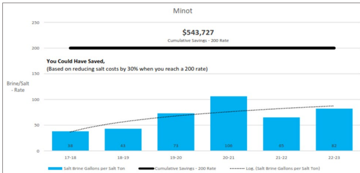
Figure 36. North Dakota calculates a brine-salt ratio for each District based on the gallons of liquid brine used versus tons of salt and generates a value of potential cost savings if more brine had been used. (Source: North Dakota DOT)
