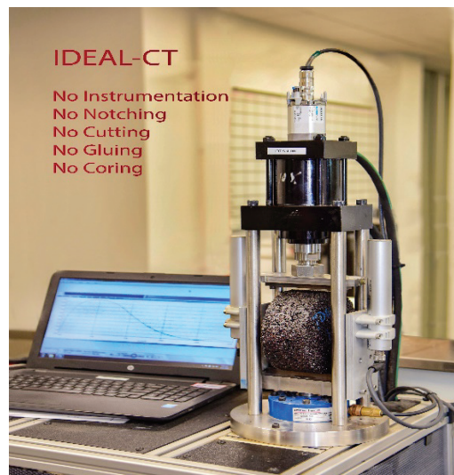
Figure 1 IDEAL-CT test setup.
